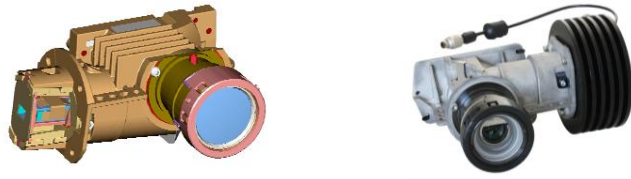
Basic LED-OM module for 0.7" XGA DMD
