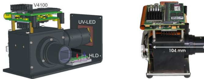
High-power LED-OM module with 388 nm UV LED for 0.7" XGA DMD
