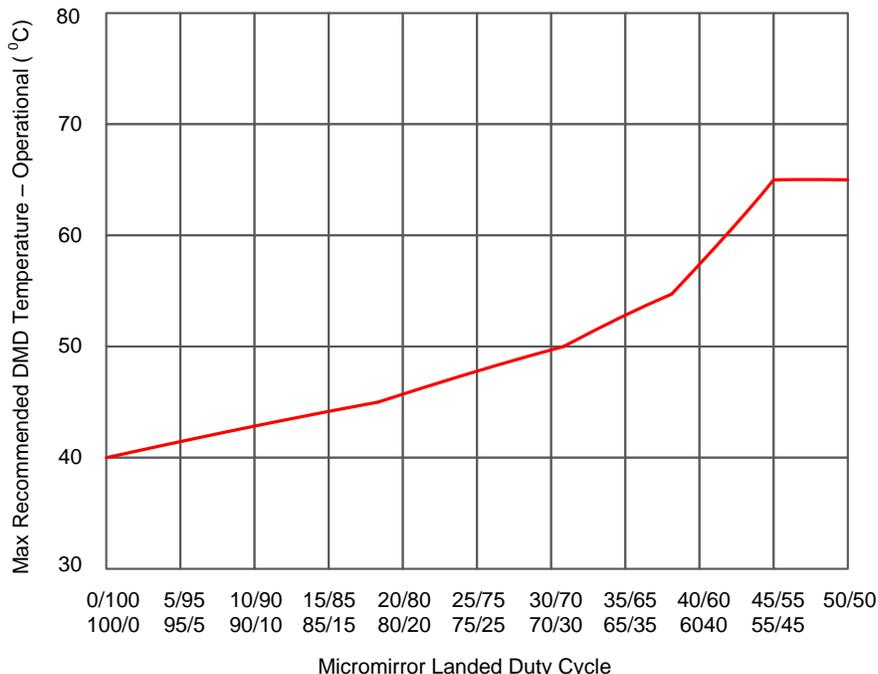
**Figure 16. Max Recommended DMD Temperature – Derating Curve**
