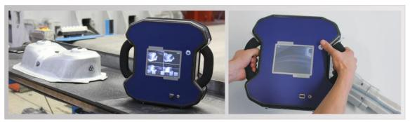
A single button trigger records a set of 4 synchronized cameras with 5 million pixels resolution. The data can be transferred online or stored for later transfer. An integrated display allows the visual image control in measuring mode.
